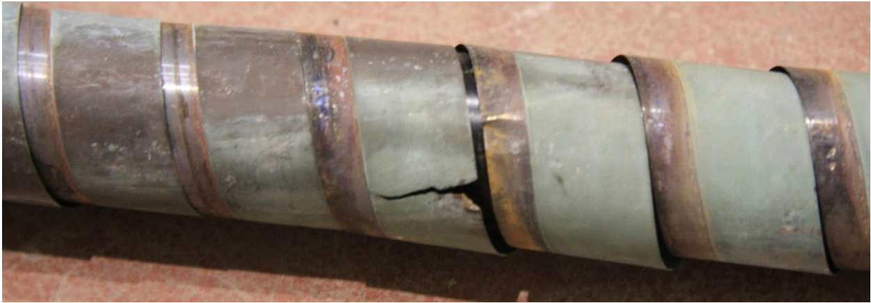
Figure 12: Tear in the Metallic Neutral
