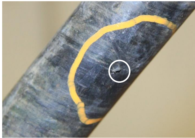
Figure 10: Small Crack in the Semicon
