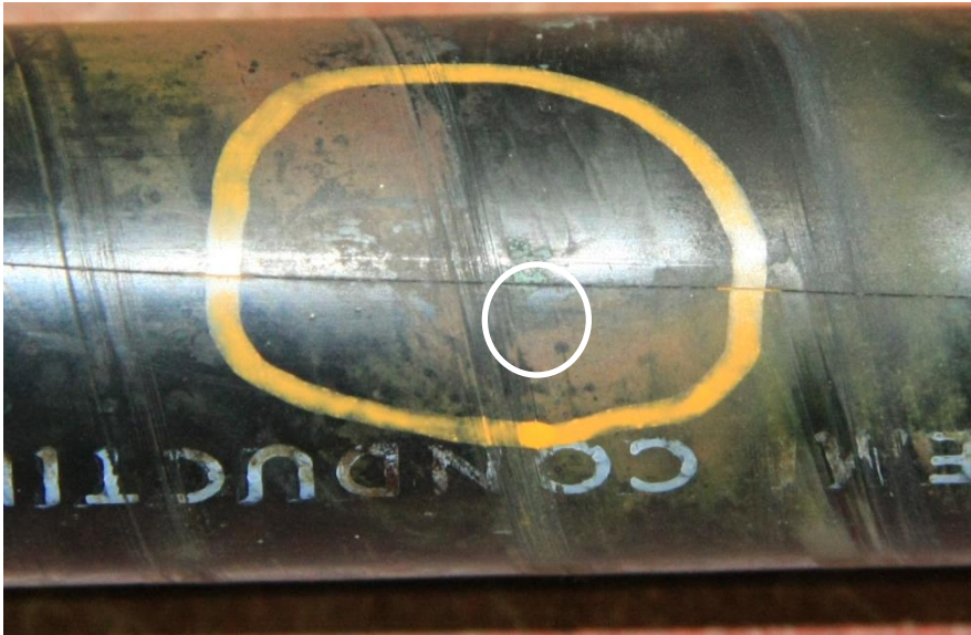
Figure 6: Minor Surface Damage to the Insulation Semicon
