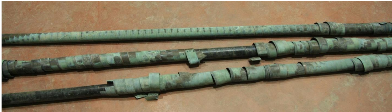
Figure 4: Condition of the Metallic Tape Neutral
